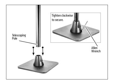
2 Attach overhead arm assembly by unscrewing the collar at the top of the pole until the metal ball side of the overhead arm assembly fits into the collar. Tighten collar clockwise to secure.
