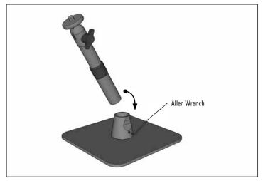
Adjust the height and angle of the mount by loosening the adjustment ring and the adjustment knob. Retighten to set.
